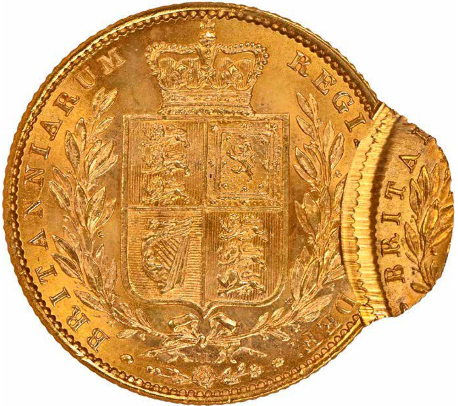
1863 Great Britain Gold Sovereign graded NGC Mint Error MS 66 - Double Struck 85% Off Center
