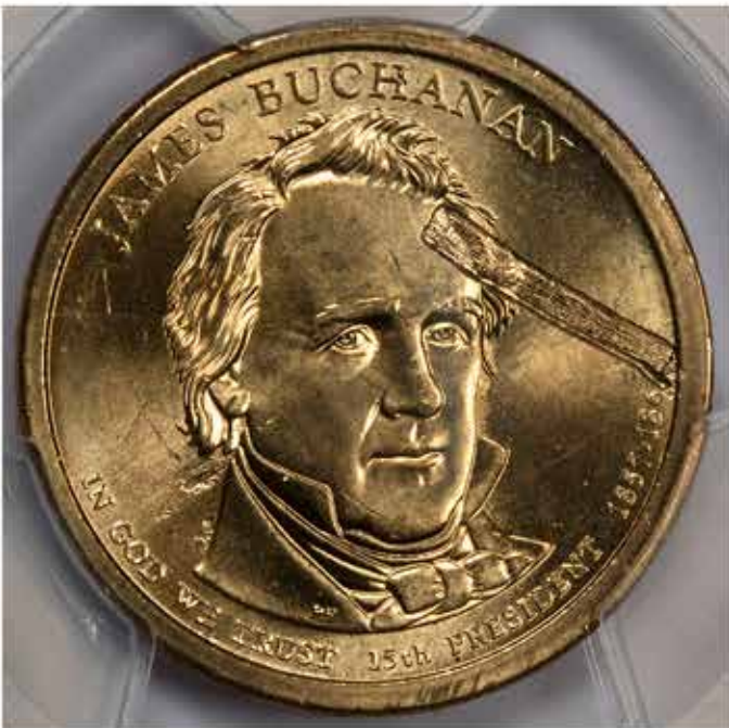
2010 PCGS SP64 Struck Thru Object (Wood) Buchanan Satin Finish Dollar Mint Error
