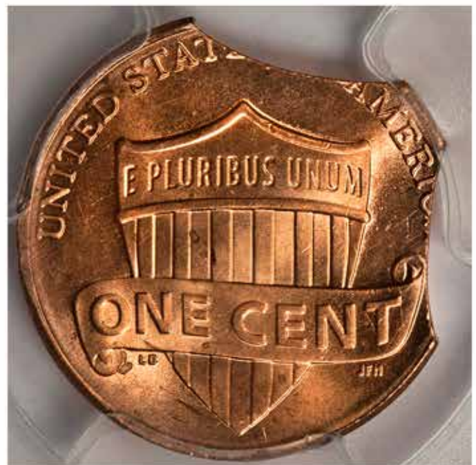
2018 PCGS MS64RD 12% Double Clipped Planchet Shield Cent Mint Error
