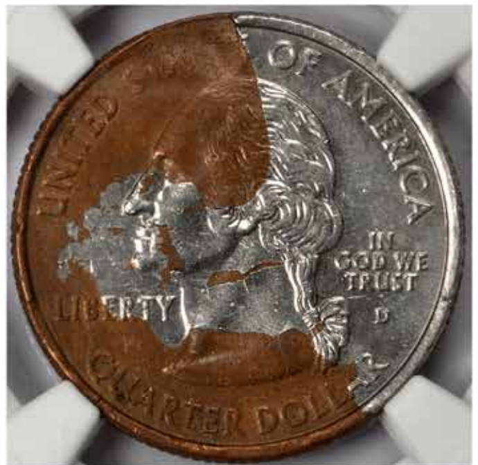
2008 D NGC MS62 Missing Partial Clad Layer Alaska Quarter Mint Error
