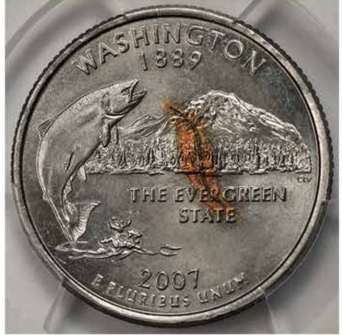
2007 PCGS MS64 Struck In Retained Steel Wire Bristle Washington State Quarter Mint Error
