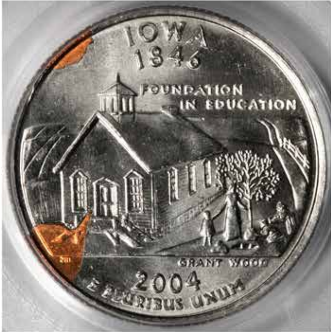
2004 D PCGS MS65 Defective Clad Layer Iowa Quarter Mint Error
