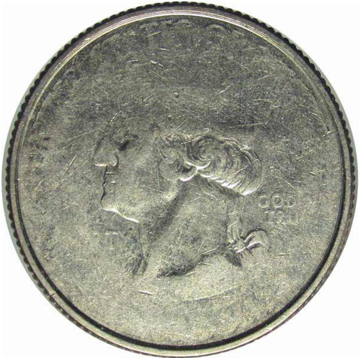
Obverse of a State Quarter struck through grease. Note the resemblance to a die adjustment strike, except the reeded edge is full. Struck thrus can also affect just one side of a coin, while a die adjustment strike will show weakness on both.
