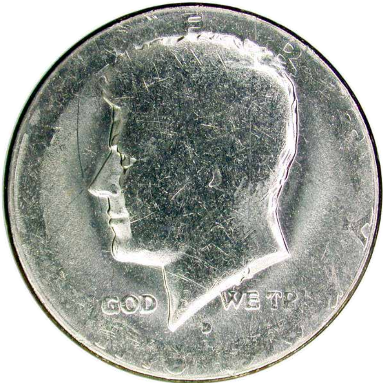
1976-D half dollar, die adjustment strike, obverse. Low pressure did not allow for all of the details of the coin to be present.
