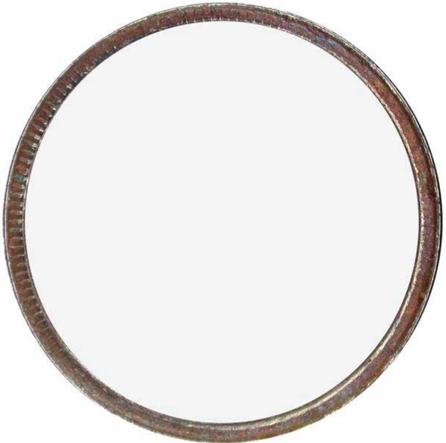
1976-D half dollar, die adjustment strike, edge view. Note that the reeding is either weak or missing from the edge of the coin.
