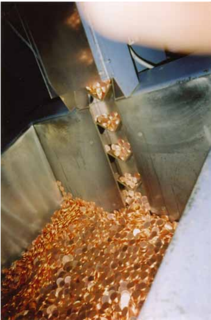
Cent Blank Planchets being fed up into Feeder Mechanism to be struck
