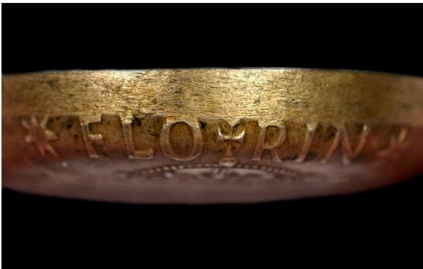
Lack of metal flow is evident on the edge of the fake 1944 Australia Florin die cap.
