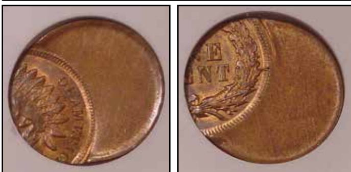
(1864-1909) Indian Cent Centered Broadstruck with a 20% Obverse Indent at K-6 and with a Reverse Retained Die Break at K-3. NGC MS 63 BN
