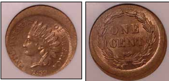
1859 Indian Cent Struck 15% Off Center at K-7 on a Type 1 Planchet. NGC MS 64
