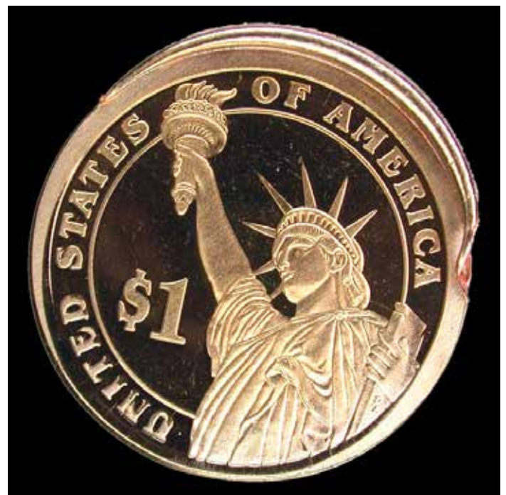
PHOTO #1b: Proof 2007-S John Adams $1 struck from horizontally misaligned dies, reverse view.
