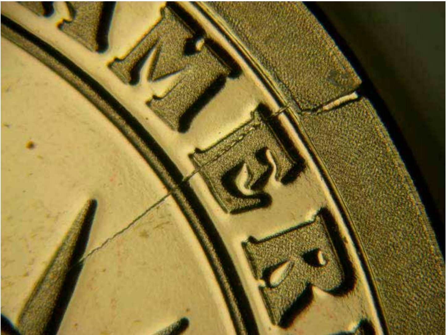
PHOTO #4a: Proof 2007-S Thomas Jefferson $1 with reverse die crack at 2:00.
