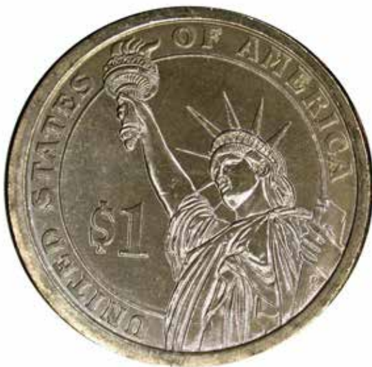
Photo #6b: Improperly annealed George Washington $1, reverse.
