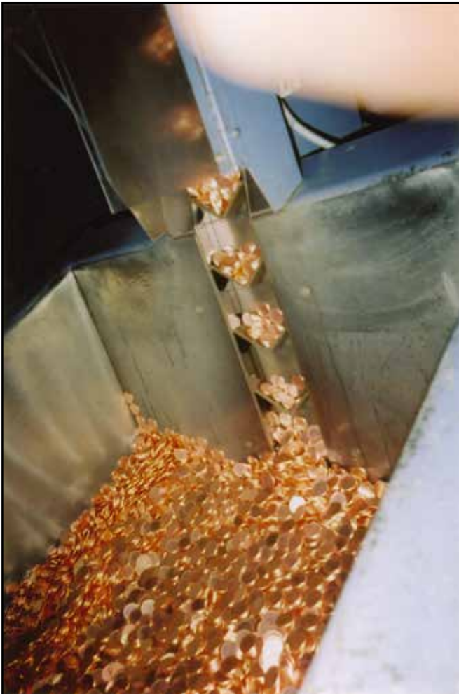
Cent Blank Planchets being fed up into Feeder Mechanism to be struck
