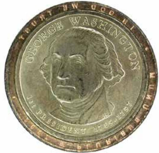
Photo #2a: Improperly spaced edge lettering. Note the wide gap between TRUST and the date preceding the date. The mint mark overlaps the start of E PLURIBUS UNUM.
