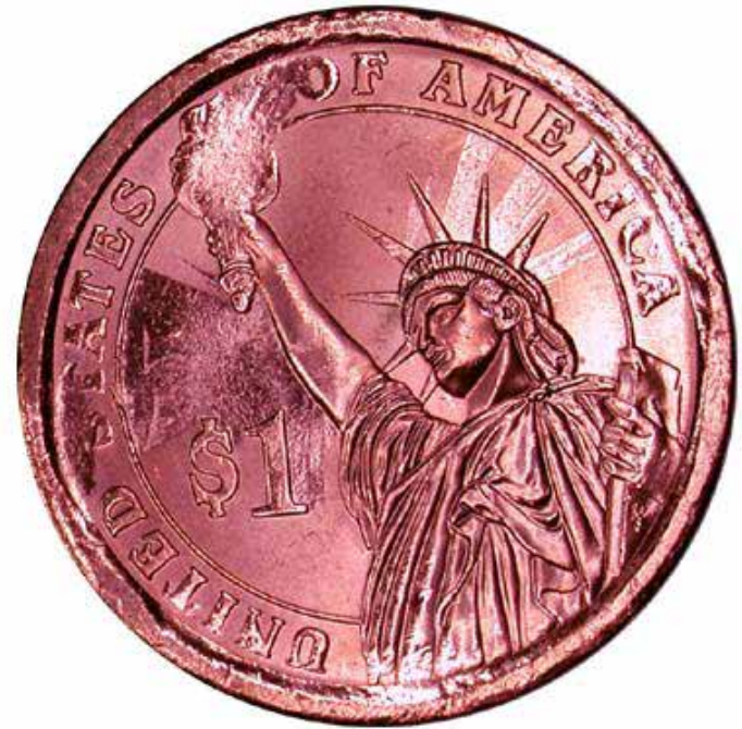
Photo #5b: Reverse missing clad layer.
