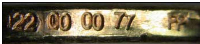
Photo #1b: Close up of overlapped doubled edge lettering.
