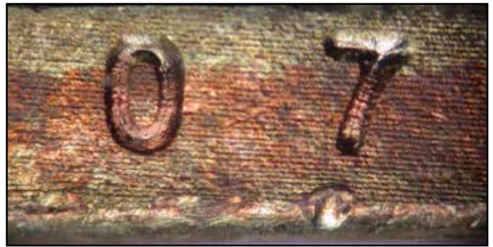
Photo #6c: A close up of the date portion of the edge and parallel lines suggesting laser etching.
