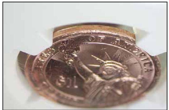
Photo #13b: Missing reverse clad layer and missing edge lettering, detail of the coin's edge as seen in the EdgeView™ Holder.
