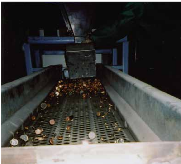
Riddler “bouncing” coins to filter out errors
