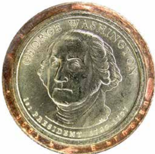
Photo #3c: Partial edge lettering. IN GOD WE TRUST and UNUM missing.
