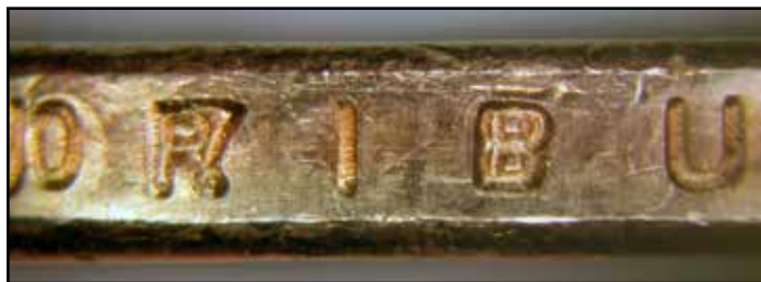
Photo #14b: A close up of the edge showing two sets of edge lettering. Here a portion of the date and mintmark, '07 P,' are seen to overlap with 'URIBU' of E PLURIBUS UNUM.
