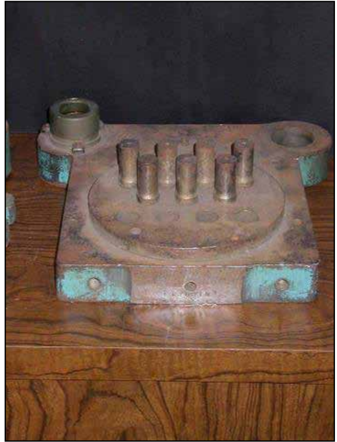
Nickel Gang Punch Press Unit from the San Francisco Mint
