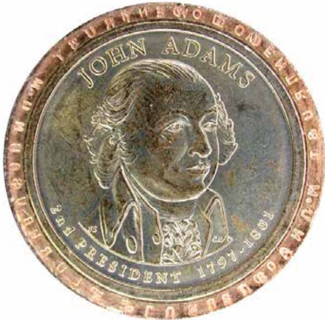
Photo #2a: Obverse with exploded edge view of 2007 P John Adams $1, showing inverted doubled edge lettering.
