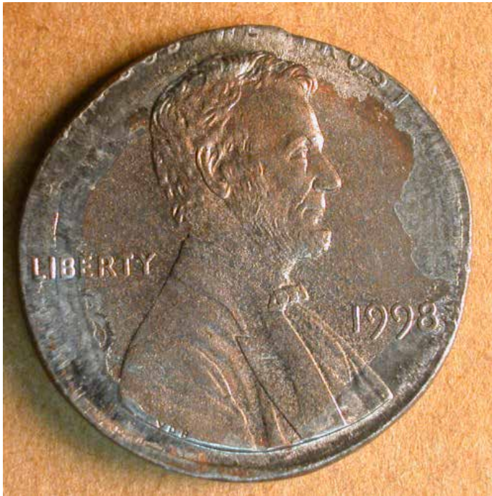
Figure 1. A 1998 cent struck on an unplated zinc planchet intended for a foreign denomination. The lack of plating is an error.
