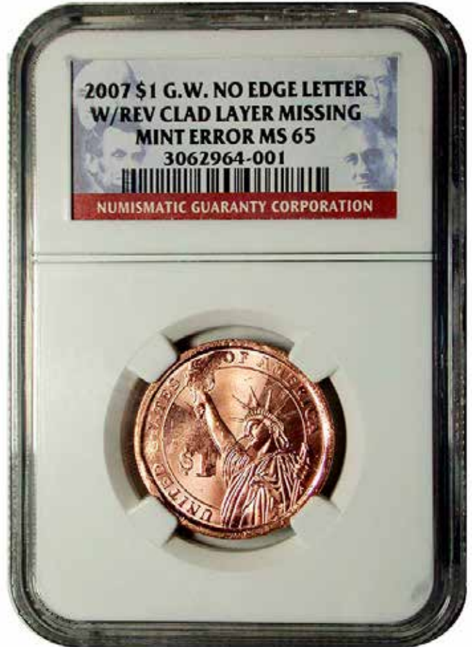
Photo #13a: Missing reverse clad layer and missing edge lettering, shown in NGC EdgeView™ Holder.
