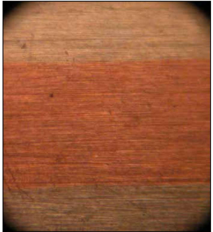
Photo 4: (File: WASHINGTON $ ALT EDGE 1) A closer view reveals the extent of the horizontal file marks and the lack of vertical ejection marks on the edge.
