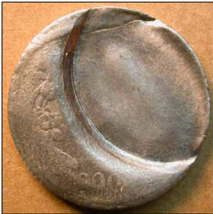
Figure 4a. Reverse face of an India 5 rupees coin, showing a 60% indent and a weak extrusion strike.
