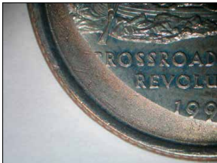
Figure 2a. Close-up of the crescentic trough.
