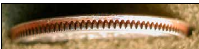
Figure 1c. Edge of the same coin photographed at the midpoint of the extrusion strike. A strong partial collar is easily seen.
