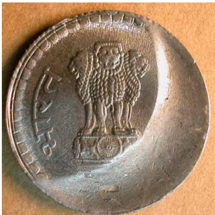
Figure 4b. Obverse face of the same coin showing an oval area of die-struck design opposite the indent, and a scooped-out, crescentic zone lying opposite the extrusion strike.
