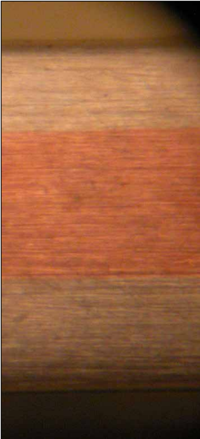
Photo 3: This is the altered Washington dollar with the edge filed down sufficiently to give the appearance of a piece that did not receive its lettered edge impression. Note the fine horizontal file marks, the rounded edge and the lack of vertical ejection marks.
